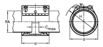
= 98 а C max with insertion band = 25 = 130 d Н = 150M (screw) = M10Nominal pressure (bar) = 16 = 110
